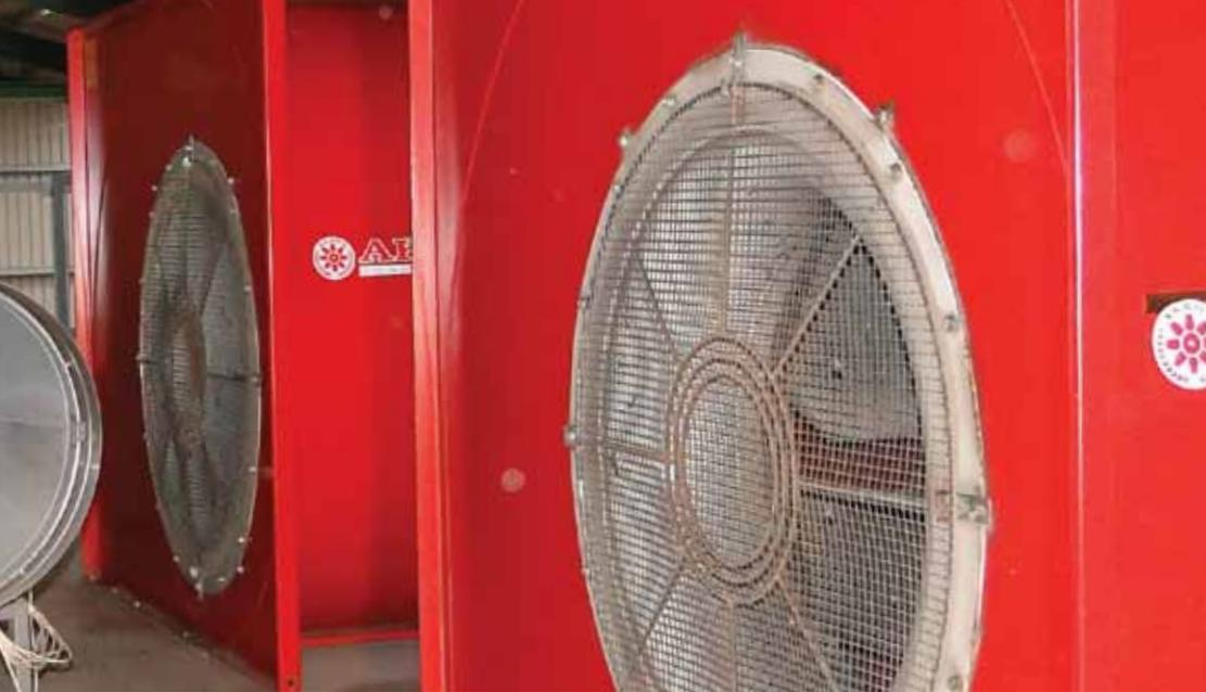
A wide range of impellers are available to give performance to suit virtually any application. All model PFD fans can be supplied with mounting feet and inlet guard. Dwindraught applications are also available.
